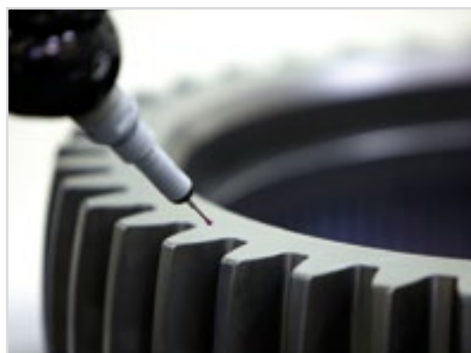
Gear inspection in CMM
